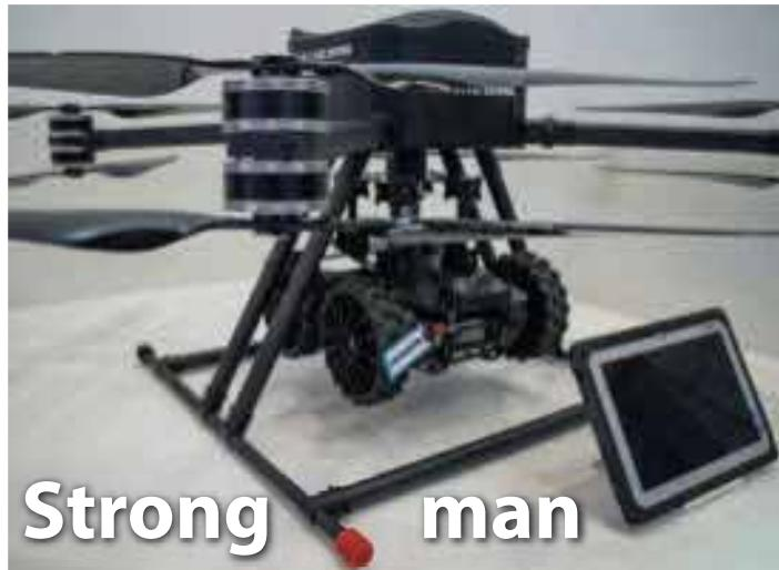
suggests, the Hercules 20 is powerful, being able to lift up to 25kg of a wide range of payloads. While lightweight and compact, it is also extremely resistant thanks to a carbon-fibre frame and anodised aluminium fasteners. The Hercules 20 stands 600mm high, but its landing gear can be removed and its arms folded for ease of transportation.
