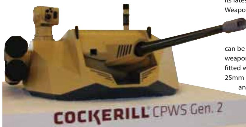
Belgian company CMI Defence (Hall 5A, Stand B267) is displaying its latest Cockerill Protected Weapon Station Generation 2 (CPWS Gen 2). This has a shell of all-welded aluminium armour and can be armed with a variety of weapons, the first example being fitted with the widely deployed 25mm M242 dual-feed cannon and a 7.62mm coaxial machine gun mounted to the left, which can be reloaded under full armour protection.
