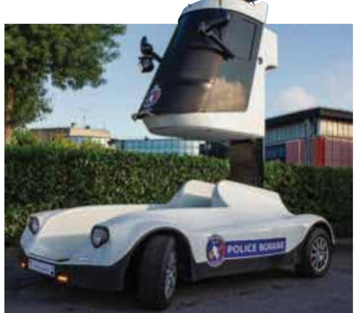
"This is a security feature to allow the driver to exit quickly in the event of an emergency," Vivier added. "In addition, the vehicle is equipped with external controls to operate the cabin without the driver inside."
