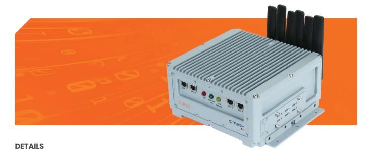
CTech MOBIoT technology increases the bandwidth by adding each communication channel's data traffic to the available band and provides fusion connectivity. In case of losing the communication links one by one, the system seamlessly keep operating without any interruption.
