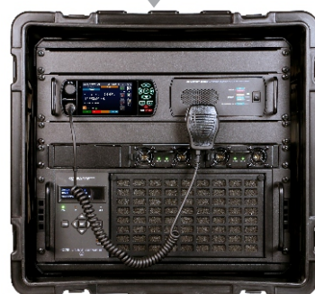
500W 4075 Transportable transmitter in 9RU 19" rack mount case
